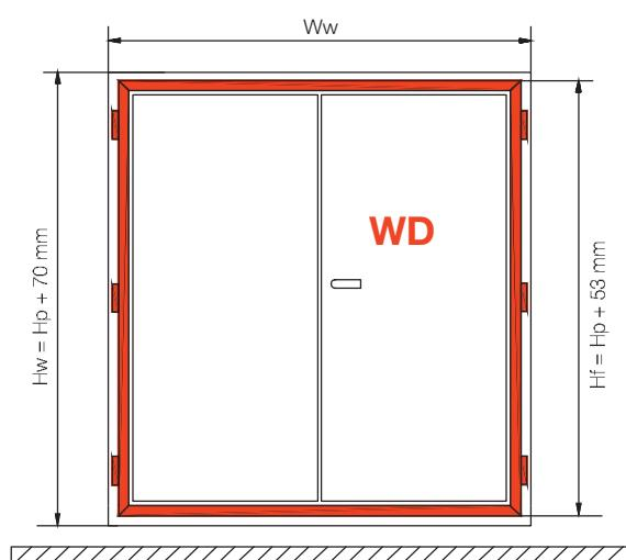
HP = Height doorpanel (max 3000mm)
